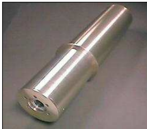
Light source showing magnesium fluoride window (vacuum adapter removed)
