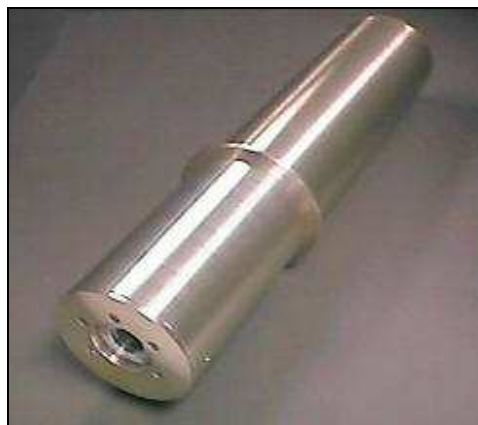
Light source showing magnesium fluoride window (vacuum adapter removed)
