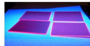
Lumogen-coated glass slides are shown fluorescing under ultraviolet illumination. The 300 nm UV light needed for the detection of SO<sub>2</sub> can be converted to visible light that regular CCD cameras are sensitive to.
