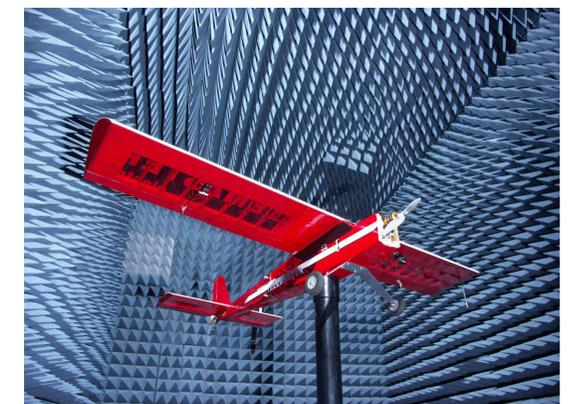
The Unmanned Aerial Vehicle in Niagara College's Anechoic chamber. The uplink and downlink are on separate frequency bands to minimize potential interference. Designed to be a portable, low-cost scientific instrumentation platform. The electric motor allows for vibration and exhaust free operation to avoid any chance of damage or contamination of the payload. The onboard computer is compatible with the majority of scientific instruments.
