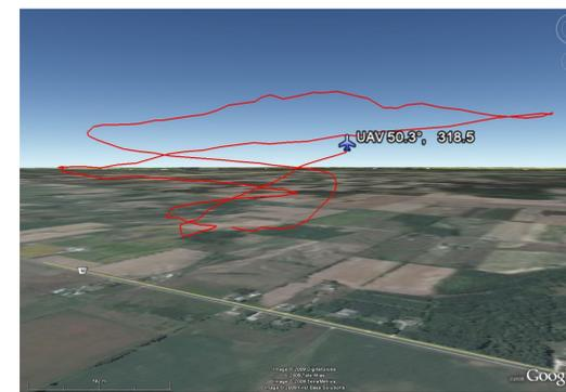
The base station for the UAV is able to track the flight in real-time using Google Earth. Commands can be sent to the UAV to alter course etc. as well as obtain SO<sub>2</sub> measurements while in flight.
