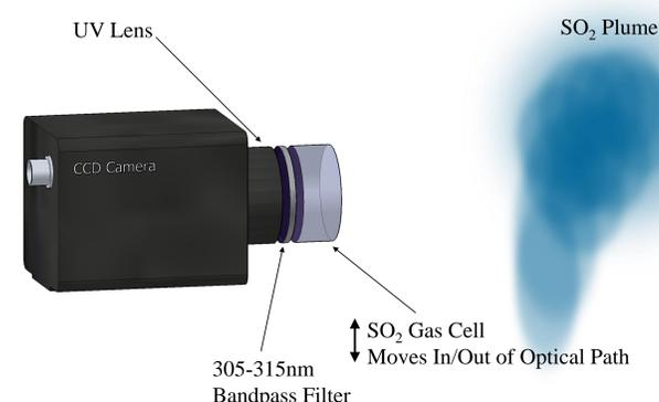
The SO<sub>2</sub> camera is based upon a gas correlation method to isolate the SO<sub>2</sub> signature in a video frame.
