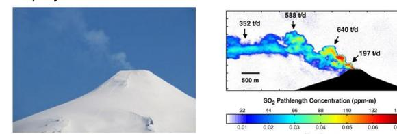
A visible picture of a volcano in Chile is shown above left, followed by a false-colour representation of SO<sub>2</sub> concentration on the right. This image exemplifies the result that will be obtained in real-time from the SO<sub>2</sub> camera.
