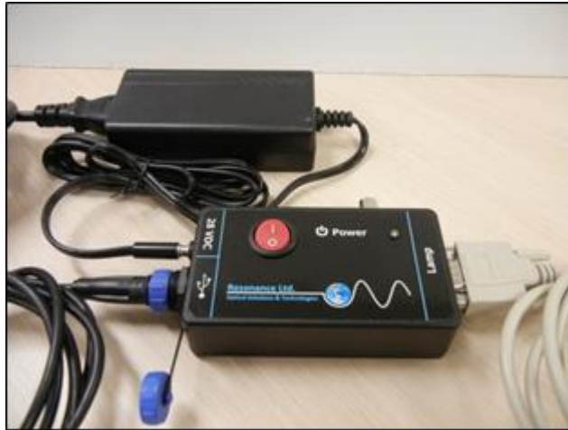
Above: Power/Data Splitter, with 24 V Input, RS-232 Telemetry, and Lamp Connector.
