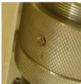
Figure 10: Exit slit focusing collar and fastening set-screw
