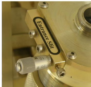
Figure 8: Slit Width Adjustment Micrometer
