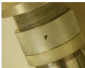
Figure 11: CCD focusing collar and fastening set-screw
