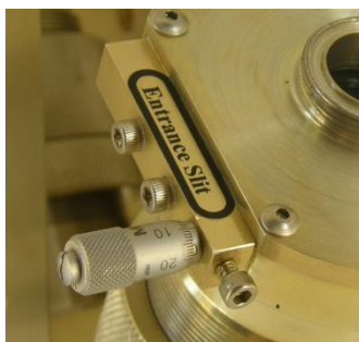
Figure 5: Slit Width Adjustment Micrometer
